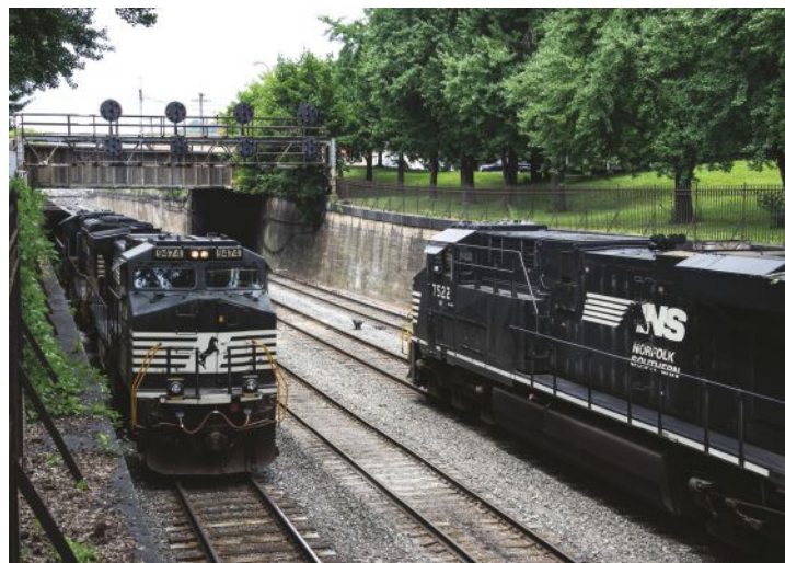
NS trains pass through Pittsburgh's North Side near a bridge that prevents passage of double-stack intermodal trains and multilevel auto racks. NS is working with PennDOT to increase rail clearance and create a high-speed double-stack corridor through the North Side.
